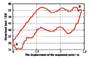
Fig. 3. the training sample data of dynamometer card image
