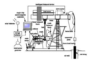
Fig. 1. Whole Structure of the Intelligent Balanced Device
